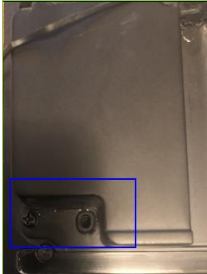
Figure 3 : Screw used to secure backplate
