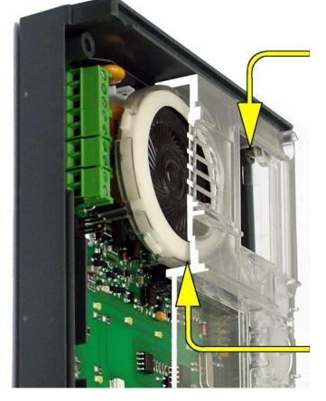
Poorly tightened screw (a squeezed wire has the same effect)
