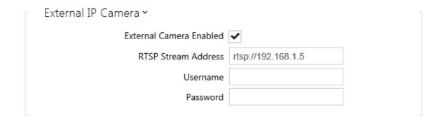
■ External camera enabled – enable RTSP stream download from the external IP camera. Complete the valid RTSP stream address or the username and password
