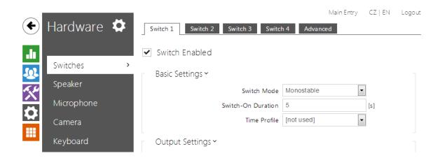
Switches provide a very flexible and efficient control of such intercom peripherals as electric door locks, lighting, additional ringing signalling, and so on.  $2N^{\otimes}$  Helios IP allo ws you to configure up to 4 (depending on model types) independent all-purpose switches.
