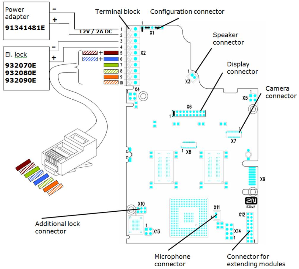
**Figure:** Description of Connectors, PCB Version 530v2
