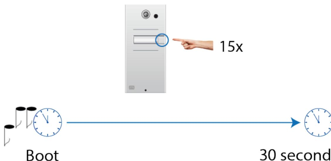
**Figure 3.3** Switching between static and dynamic IP address
