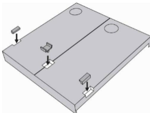
5. Install blank modules on the unused side holes as shown in Figure previous step.
