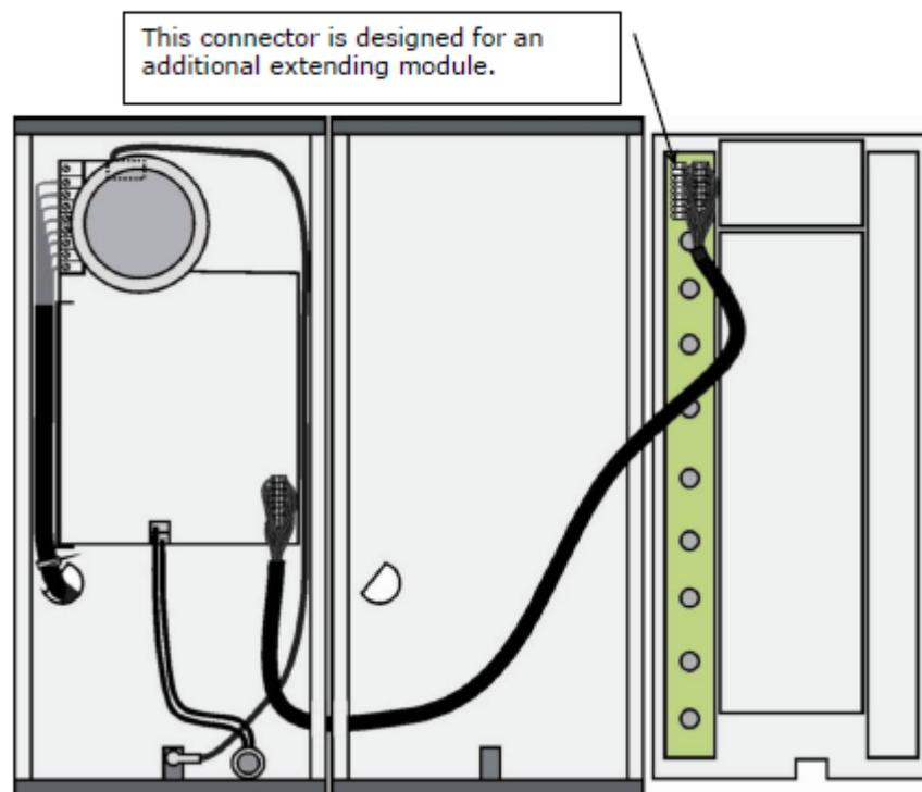
**Figure:** Connection of One-Row-Button Extending Modules
