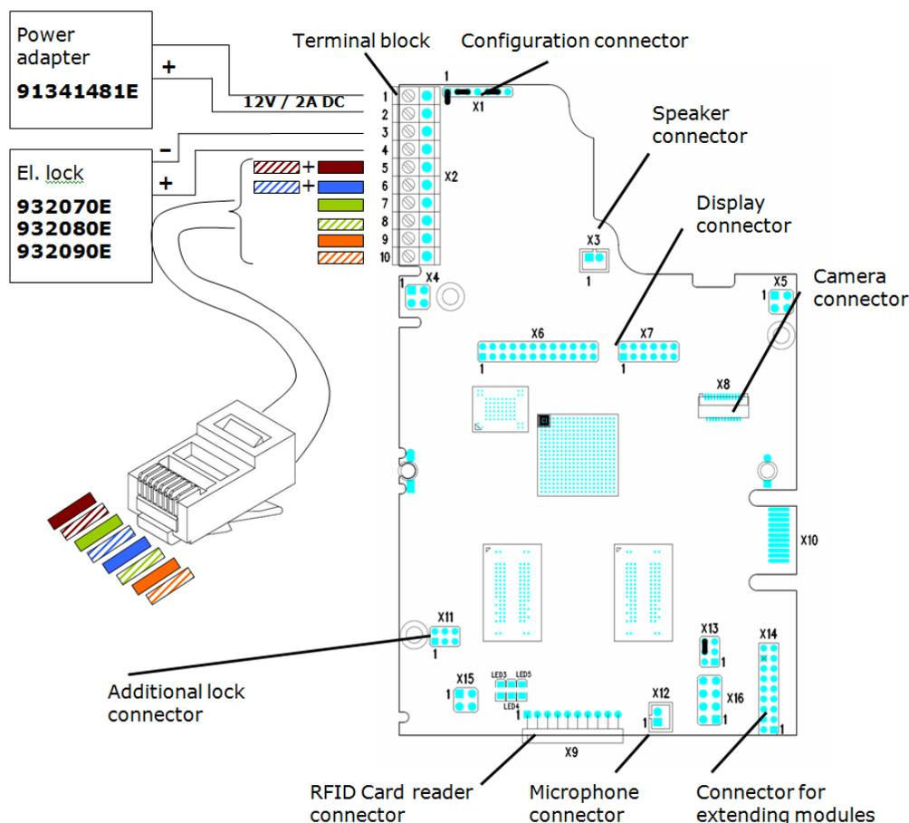
**Figure:** Description of Connectors, PCB Versions 535v5
