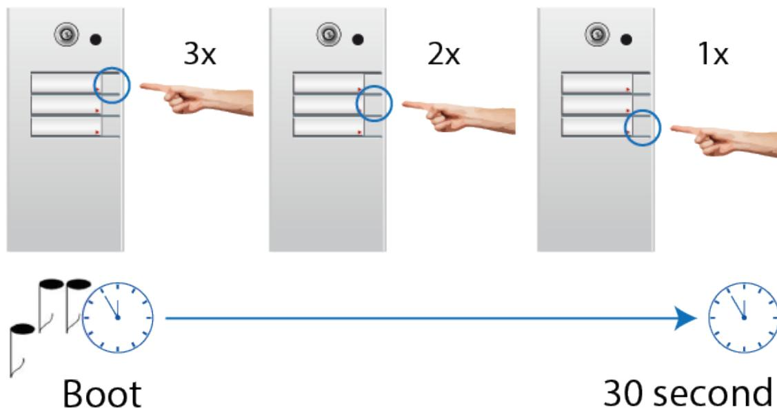
**Figure 3.1** Switching to static IP address
