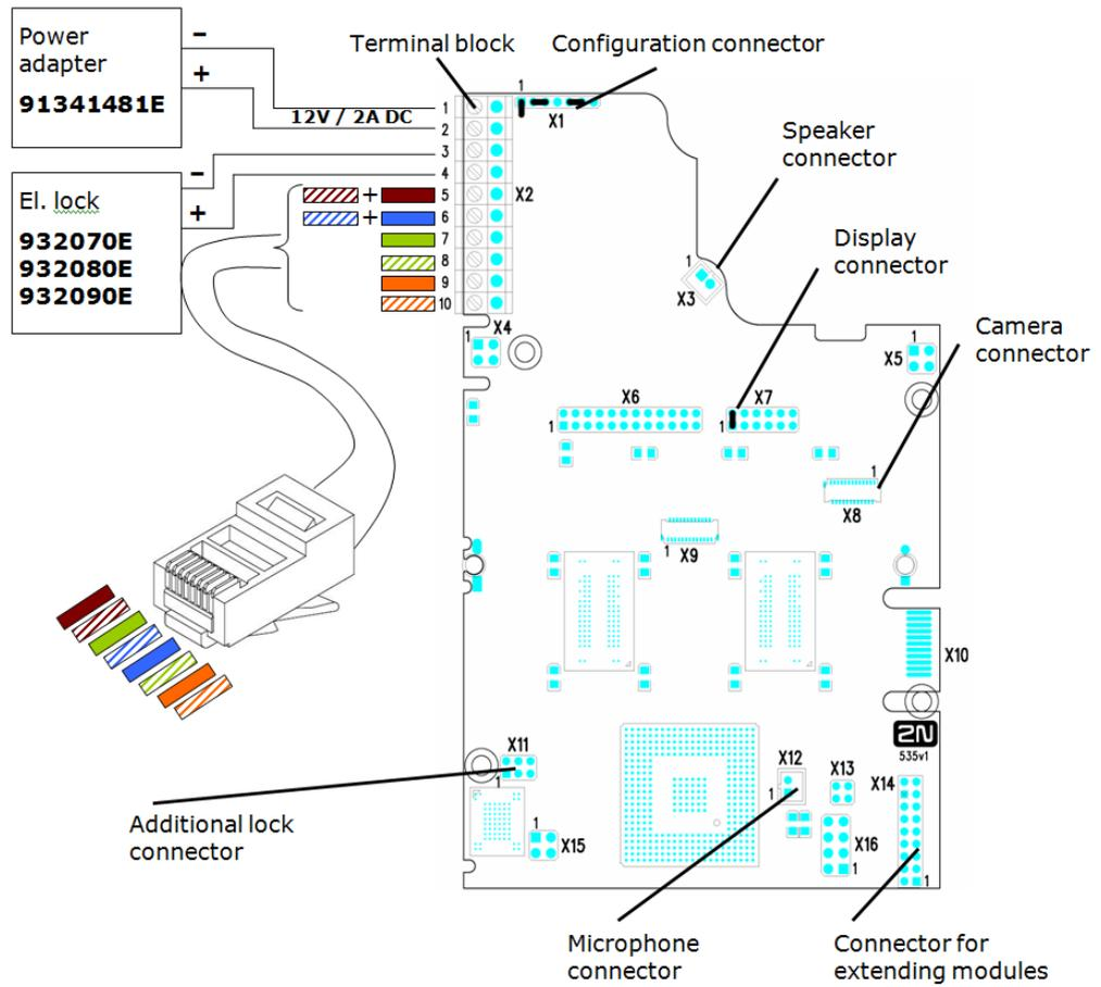
**Figure:** Description of Connectors, PCB Versions 535v1, 535v2
