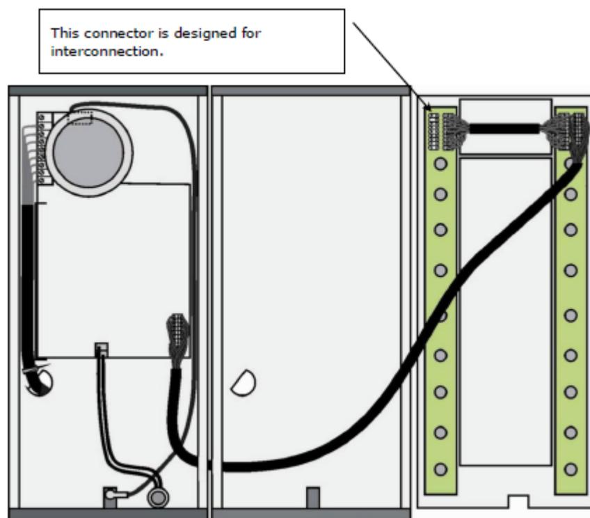
**Figure 2.16** Connection of Two-Button-Row Extending Module
