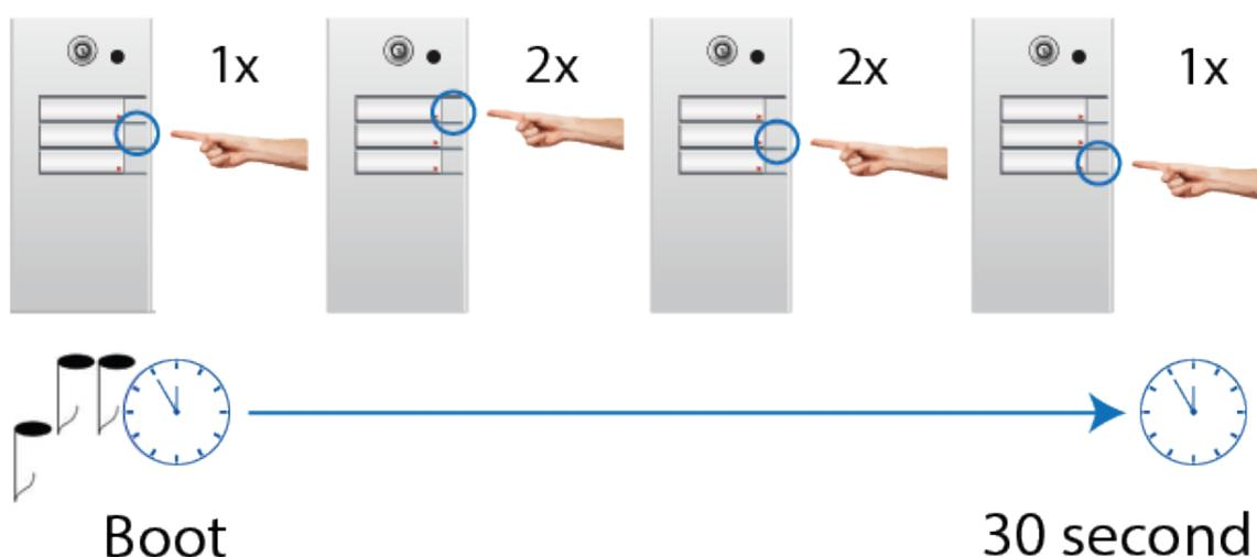
**Figure 3.2** Switching to dynamic IP address
