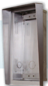
Roof & box for masonry fitting for 1 module Mask: 129 x 240 x 41 mm Hole: 110 x 220 x 50 mm (Ord. num. 9135361E)
