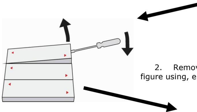
2. Remove the name plates as shown in the figure using, e.g., a screw driver.
