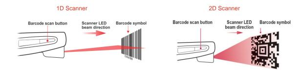
When a beep sounds to indicate a successful scan and the red light turns off, release the scan button. If you wish, you can change the barcode reader sound.
