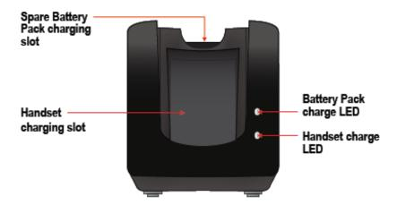
The Dual charger has two LEDs. The top LED indicates the charging status of the Battery Pack in the rear bay. The bottom LED indicates whether or not the handset is properly seated in the front charging bay. The battery status icon on the handset indicates the charging status of the Battery Packs.
