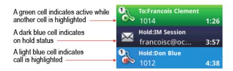
When a cell is highlighted, softkeys display that you can press to affect that call while other cells remain unaffected. Use the ▲ and ▼ and OK navigation keys to scroll to, highlight, and select cells.
