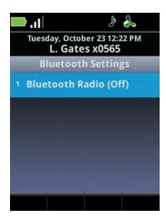
2 Select **Bluetooth Radio** and turn Bluetooth on. When Bluetooth is turned on, the Bluetooth icon ( ) displays in the Status Bar.
