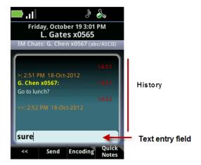
When a new IM chat window opens, you can type a new message. The default entry mode is alphabetic. Use the *Encoding* softkey for entering numbers and other characters. Use the *Quick Notes* softkey to enter preprogrammed messages. A message can be up to 128 characters in length. Once you have finished typing your message, press **OK** to send.
