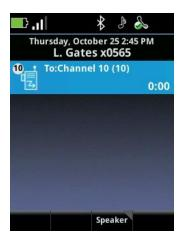
When you release the *Talk* button, the handset enters a ten-second wait period during which the channel is open to receive or send additional broadcasts. If no activity occurs within the wait period, the cell is closed. A waiting cell displays an orange call icon.
