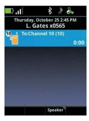
The wait period keeps the channel open and gives any handset subscribed to that channel time to join the conversation. To open a different channel or to send a new broadcast within the wait period, end the wait period on the current channel by pressing the **End** key.
