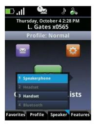
When a softkey menu displays, there are two ways to choose a menu item. Use the ▲ and ▼ navigation keys to scroll through the shortcut menu and press the **OK** key. Or, press the number of the option on the keypad. Grayed options are not available.
