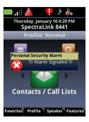
When you are in an alarm state, the alerting ring tone or vibration can be turned off by selecting the **Silence alarm** option on the Features softkey menu. Only the audio/vibration is stopped. The alarm state will continue until cleared. The flashing LED continues until the alarm state is cleared.
