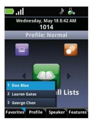
You can select a name from the speed dial menu or use the keypad to press a speed-dial index number. The call is placed immediately.
