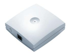
The Spectralink DECT Repeater is a building block used to extend the wireless coverage area within a Spectralink DECT network. The DECT Repeater provides a larger geographical spread of the traffic channels and increases the coverage area. But because it does not increase the number of traffic channels available, the DECT Repeater is mainly used in areas with limited traffic.
